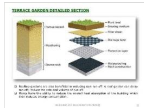
Figure 13: Terrace Garden Detailed Section and Ventilation Systems
